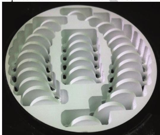
Figure 1: Milled zirconia disc specimens.
