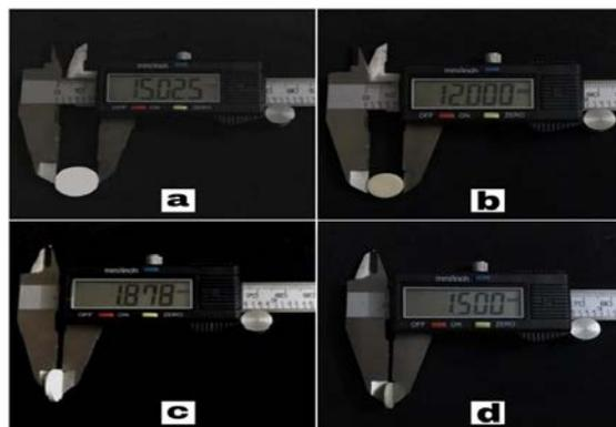
Figure 2: Digital caliper measuring (a&b) diameter and (c&d) thickness of specimens before and after sintering respectively.
