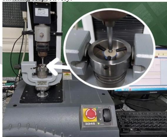
Figure 3: Biaxial flexural strength test using universal testing machine.
