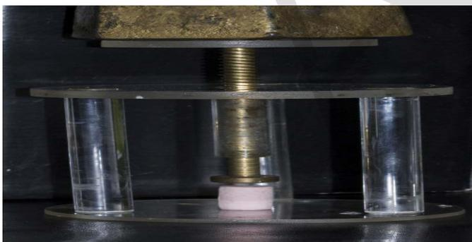
**Figure (2):** The shear force was applied parallel to the interface of the bonding surfaces.
