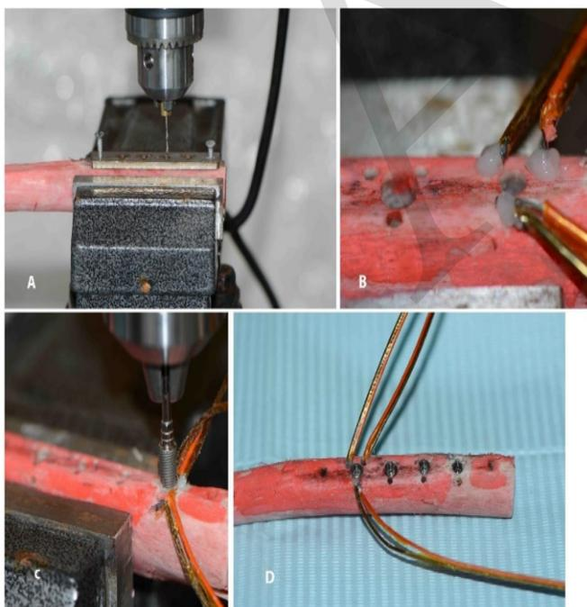
**Figure (3):** (A) Preparing the thermocouple channels (B) Application of the insulating material, (C, D) show the implant insertion.
