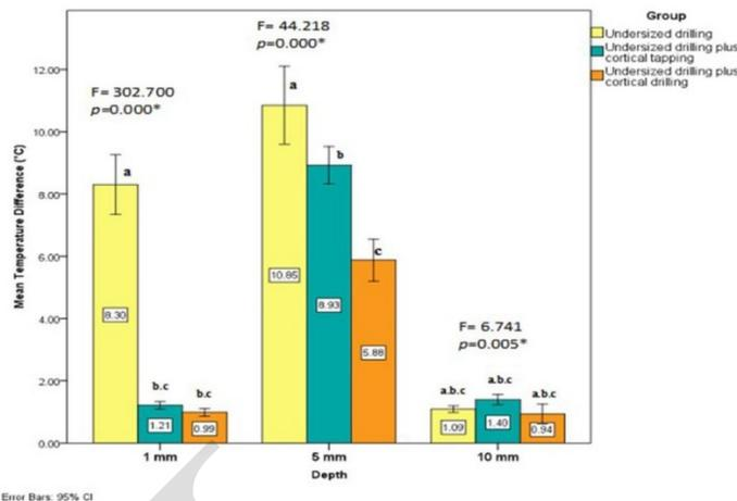
**Figure (5):** Clustered bar chart with 95% CI of the mean of temperature difference (°C) at different osteotomy depths during implant insertion for different drilling techniques studied.
