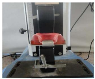
**Figure (6):** The universal testing machine dislodging the overdenture.
