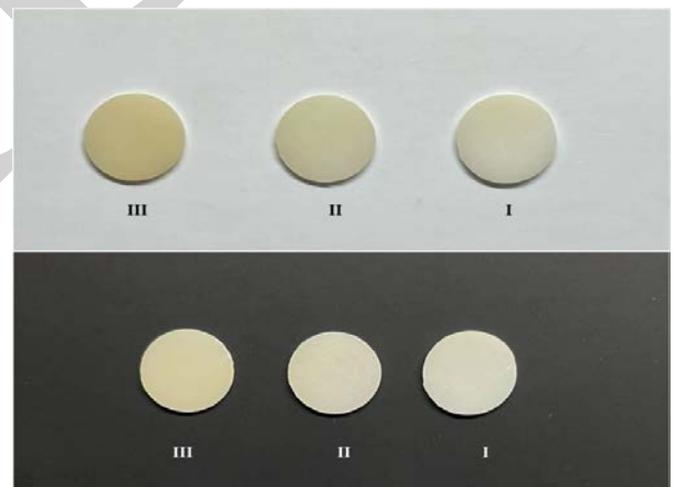
**Figure (2):** Transparency Parameter (TP) at different parts of specimens of different thicknesses tested on white and black paper
