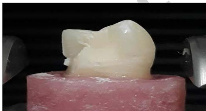
**Figure 4:** Fractured inlay restoration from group A showing catastrophic failure
