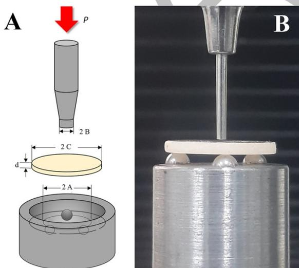
**Figure 3:** BFS testing method by piston-on-three-ball test following ISO 6872.
