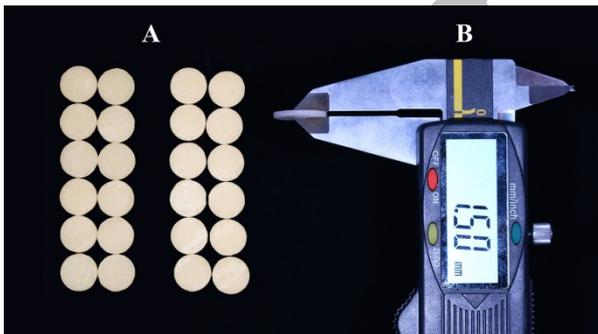
**Figure 2:** (A): 12 Pressed and 12 Re-pressed Celtra® Press ceramic specimens. (B): Thickness of polished pressed ceramic specimen.
