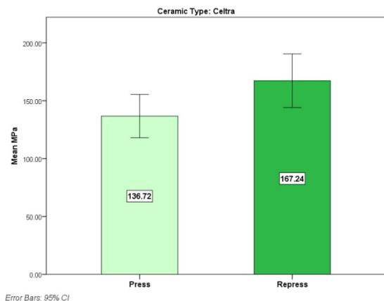
Figure 4: BFS of pressed and re-pressed specimens.
