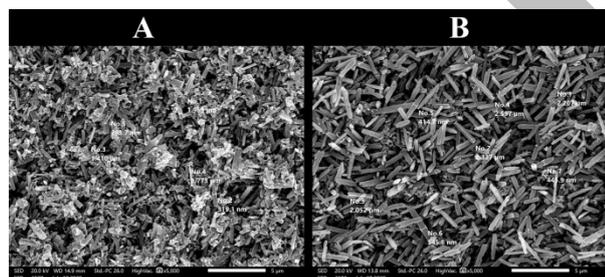
Figure6: Scanning electron microscope photomicrograph (5000X) after etching. (A): Pressed Celtra® Press specimen. (B): Re-pressed Celtra® Press specimen.
