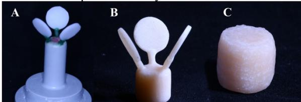
**Figure 1:** (A): CAD-CAM milled wax specimens after spruing. (B): 3 Celtra® Press pressed ceramic specimens. (C): Pressed Celtra® Press ingot used in repressing after adjustments.
