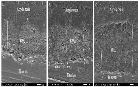
**Figure 3:** SEM images of cross sections of coatings done by applying 10V (A), 30V (B), and 50V (C).
