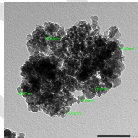
**Figure 1:** TEM image of the prepared BAG nano-powder.
