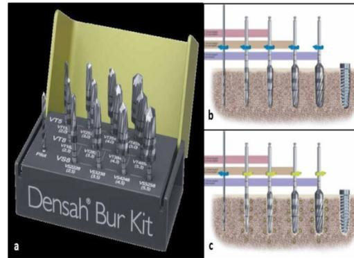
**Figure 2:** a: The complete kit of 13 Densah drills. b: The Densah drills will cut when run in a clockwise direction at 800-1,500rpm. c: Running the drills counter-clockwise produces the densification effect
