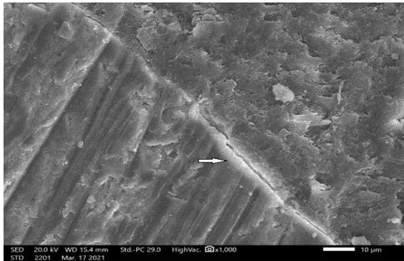
**Figure (1B):** Scanning electron micrograph of AgNPs group showing a straight, uniform line denoting the tooth surface-sealant interface. Note the definite white zone at the interface (white arrow) (Mag.x 1000)
