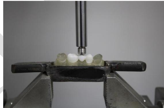
**Figure 4:** Custom-made jig with the specimen during testing.
