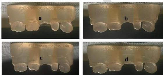
**Figure 1:** 3D printed epoxy resin models with different proximal finish line thickness (a: 0.4mm; b:0.8mm; c: 1mm; d:1.2 mm).
