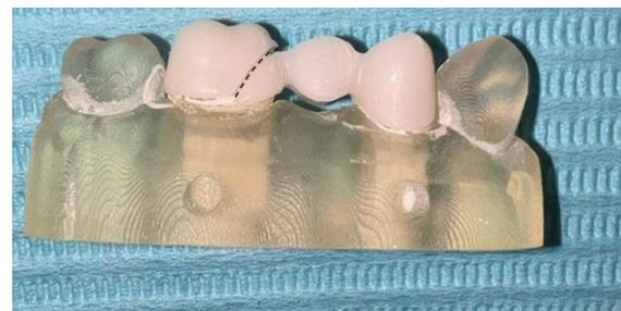
**Figure 5:** Group I (1 specimen) showing the buccal crack extension.
