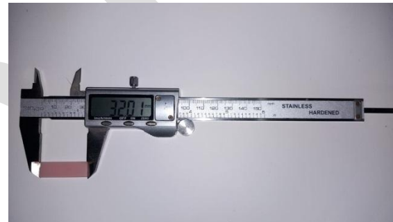
Fig. 4: length measuring using digital caliper
