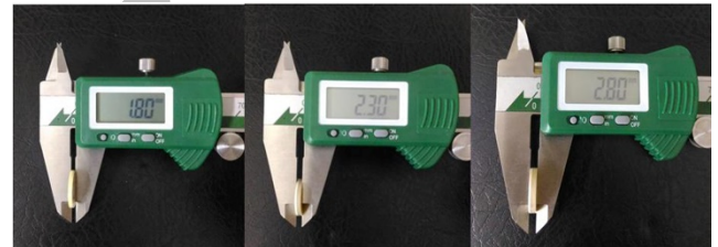
Figure 2: Measurement of the specimens after veneering using digital caliper.
