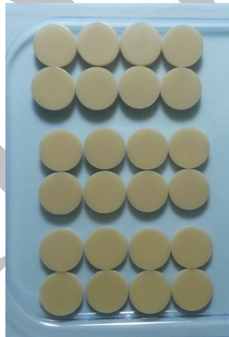
Figure 3: PEEK specimens veneered by composite.
