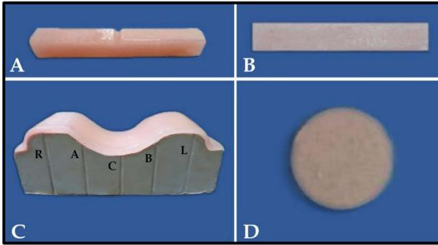
**Figure 2:** (A): Showing impact strength test specimen. (B): Showing flexural strength test specimen. (C): Showing the sectional stone cast with five locations used for measurement of warpage. (D): Showing the specimen for testing the amount of residual monomer.
