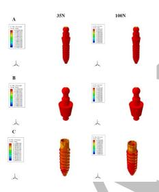
**Figure 3:** Von Mises stress patterns under 35N and 100N vertical load (**A**) 1-piece implant, (**B**) Abutment of 2-piece implant, (**C**) Fixture of 2-piece implant.
