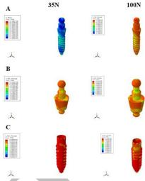
**Figure 5:** Von Mises stress patterns under 35N and 100N Oblique load (**A**) 1-piece implant, (**B**) Abutment of 2-piece implant, (**C**) Fixture of 2-piece implant.
