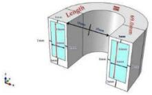
**Figure 1:** Dimensions of the model of the mandible. It was deemed unnecessary to construct a model of the
