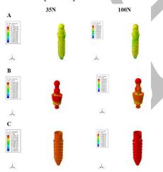
**Figure 4:** Von Mises stress patterns under 35N and 100N Horizontal load (**A**) 1-piece implant, (**B**) Abutment of 2-piece implant, (**C**) Fixture of 2-piece implant.
