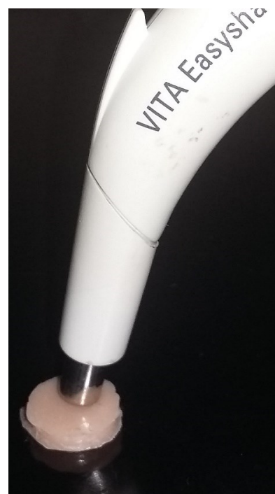
Figure 1: Color reading using VITA Easy Shade.
