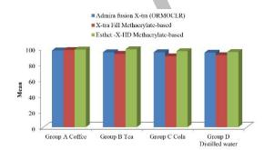
Figure (2): Comparison between opacity in different materials and group after 28 days.
