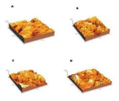
**Figure (4):** Admira fusion X tra 3-D image of surface after staining with (A) coffee, (B) tea, (C) cola, (D) distilled water.
